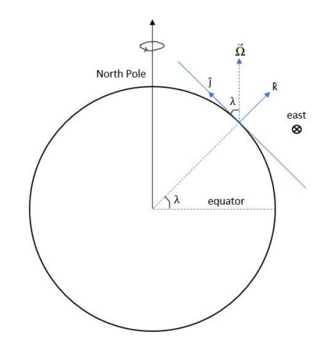
Momentum equation for inviscid fluid in a rotating frame of reference:  $\frac{D\vec{u}}{Dt} + \nabla \vec{p} = -2\vec{\Omega} \times \vec{u} + \vec{F}_{ext}$  where  $\vec{u} = u\hat{i} + v\hat{j} + w\hat{k}$
