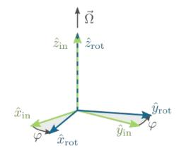
$$\frac{d\vec{u}}{dt} = \left(\frac{\partial u}{\partial t}\hat{i} + \frac{\partial v}{\partial t}\hat{j} + \frac{\partial w}{\partial t}\hat{k}\right) + \left(u\frac{d\hat{i}}{dt} + v\frac{d\hat{j}}{dt} + w\frac{d\hat{k}}{dt}\right) = \left(\frac{\partial u}{\partial t}\hat{i} + \frac{\partial v}{\partial t}\hat{j} + \frac{\partial w}{\partial t}\hat{k}\right) + \left(u(\vec{\Omega} \times \hat{i}) + v(\vec{\Omega} \times \hat{j}) + w(\vec{\Omega} \times \hat{k})\right)$$
