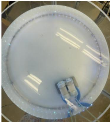
For this project, we conducted experiments in both a still and rotating tank. The still tank experiments provided a way for us to familiarize ourselves with the procedure, equipment, and underlying concepts. They also allowed us to explore the relationship between the various parameters involved with the pressurized system.
