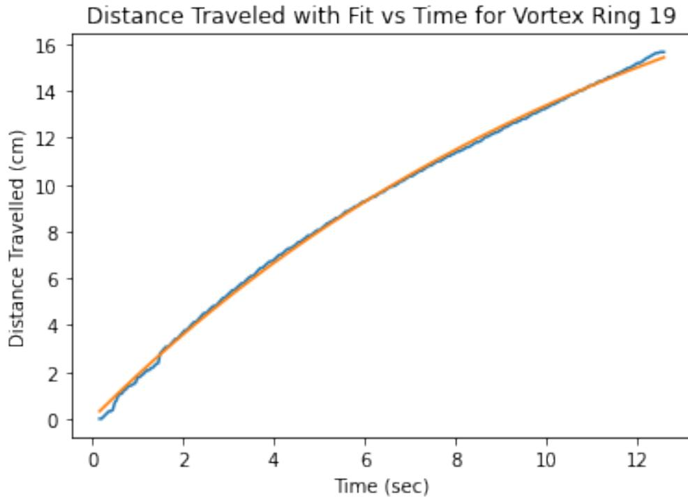
Figure 6: The distance travelled by vortex ring number 19 plotted against the time. The distance travelled is excellently fit by the linear drag model.
