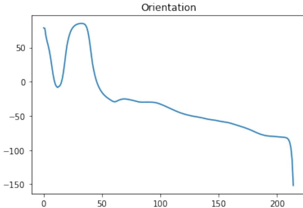
Figure 8: A sample from all of the orientation graphs from the vortex ring data. A general linear downward trend can be observed with the exceptions of the beginning and end. These are consequences of the ellipse approaching the shape of a circle, and the orientation of the ellipse allows for inaccurate orientations.
