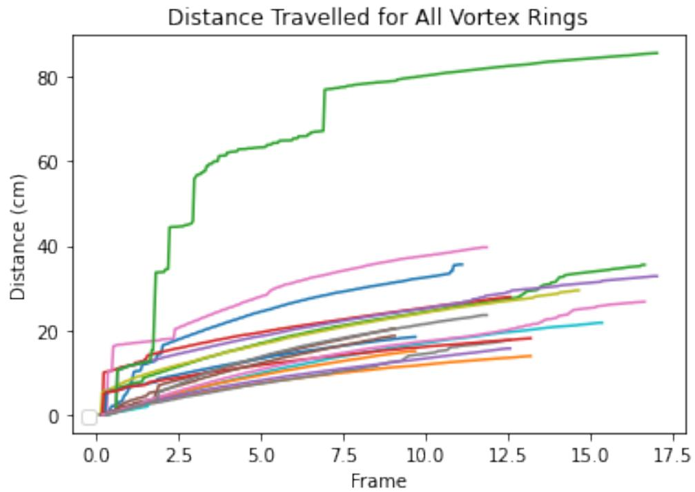
Figure 7: All of the distances travelled by vortex rings are presented above. All having similar curves representing the displacement solution to the linear drag model. It can be noted the green graph having rigged jumps demonstrates further need to improve the tracking code.
