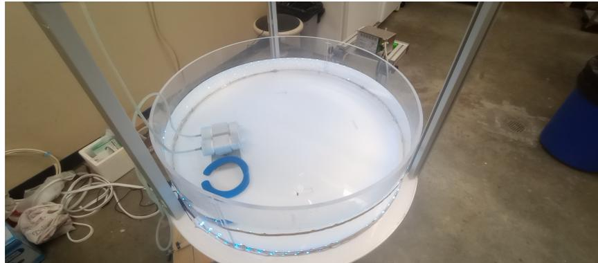
Figure 2: The image above shows the tank with the positioning of the two vortex cannons. This is the center stage for our experiment
