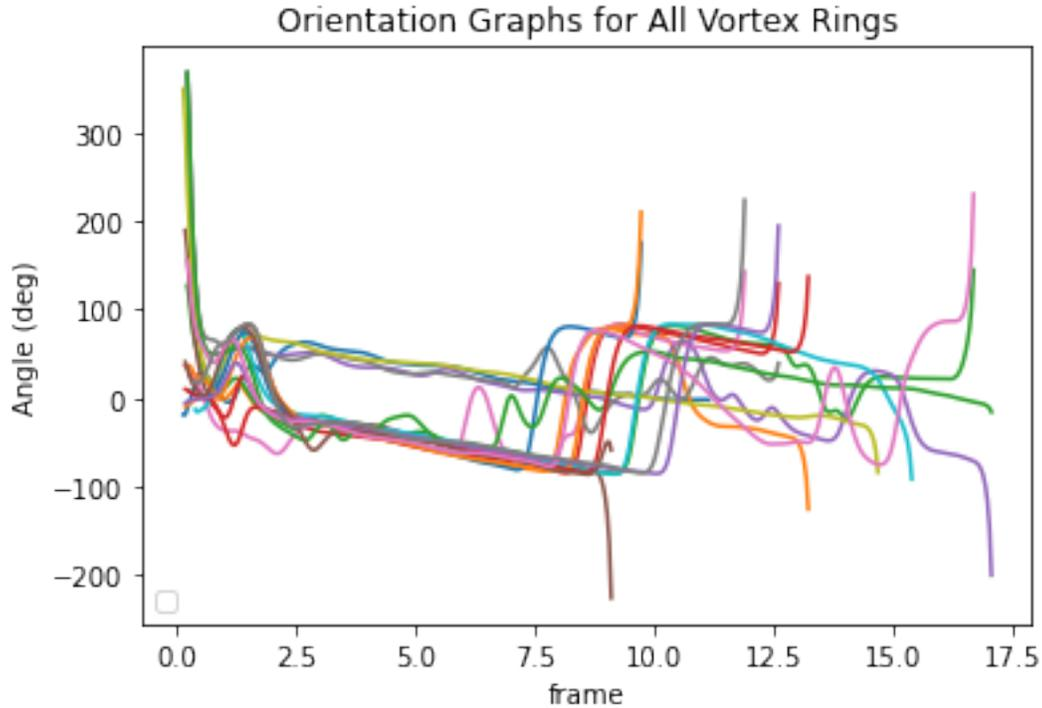
Figure 9: The collection of all orientation graphs. Many of the graphs can be seen having the general downward linear slope mentioned before.
